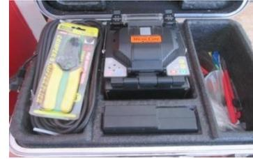
Gambar 8. *Fusion Splicer Type 39* (Sumber PT. Telkom Ternate)
